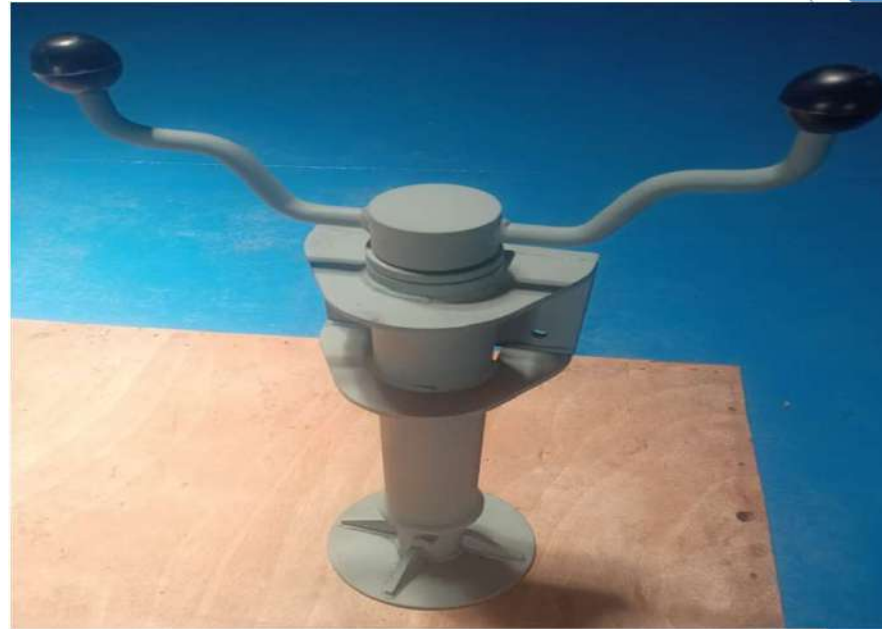
Screw Jack Assembly Process : Cutting + Machining + Welding + Inspection
